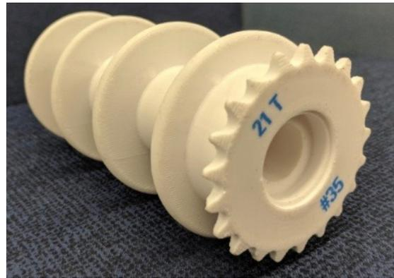
"We chose the [Rize One](#) 3D printer to print the part due to Rize's isotropic part strength and ink marking capability," said Jackie. "Labeling was printed directly onto the end of the sprocket part to indicate which chain the students need to use to use with that sprocket. This avoided any confusion and potential malfunction."
